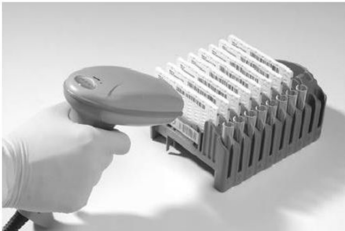
Figure 3. VITEK 2 Compact Cassette Loaded with 10 Cards and Suspension Tubes and Bar Code Scanner for Data Entry.
